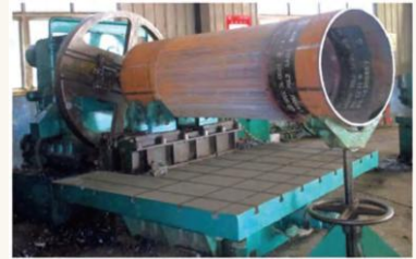
Pipe rolling & expanding
